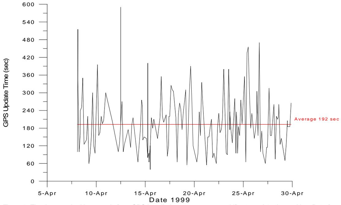
Figure 3. The time required in seconds for a GPS installed on an open ocean drifter to update the position. Data from the German Drifter 2295 WMO No 65594.
