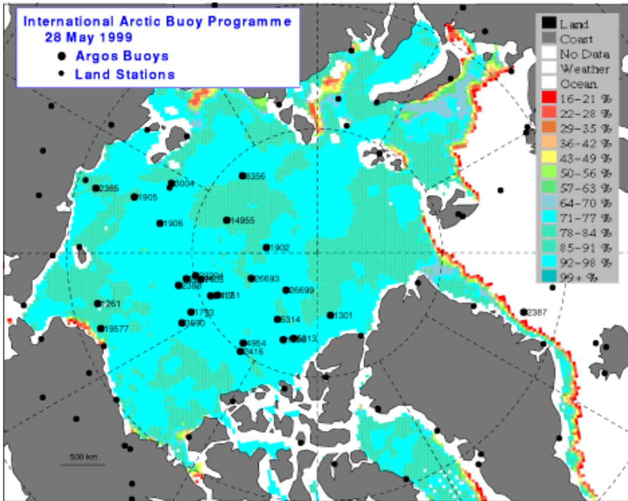
Figure 2. Buoy array on 28 May 1999. The ice concentration as analyzed by NCEP is also shown.
