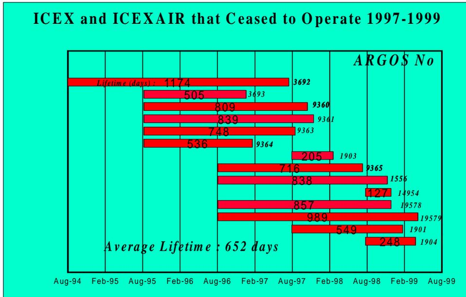
Figure 2. Gantt-diagram showing the operational periods of all ICEX and ICEXAIRs deployed under the IABP that ceased to operate 1997-1999. (Data from IABP website at <http://www.iabp.washington.edu>)
